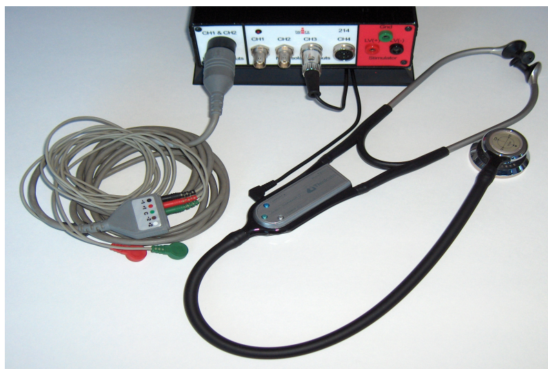
Figure HH-9-S3: The ECG cable and electronic stethoscope connected to an IWX/214.
